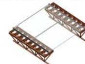
CONCEPT OF THE GLASS PLATES - STEEL BB.CC. BEAMS SYSTEM
